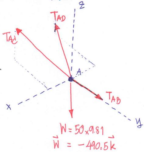
$$\vec{T}_{AD} = -0.23 \vec{T}_{AD} \vec{i} - 0.92 \vec{T}_{AD} \vec{j} + 0.31 \vec{T}_{AD} \vec{k}$$
